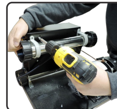
Fig. 4 - Install the booster heater to the control box utilizing the heater clamps. Tighten the heater clamps using the washers and screws provided. *See instructions provided with booster heater.
